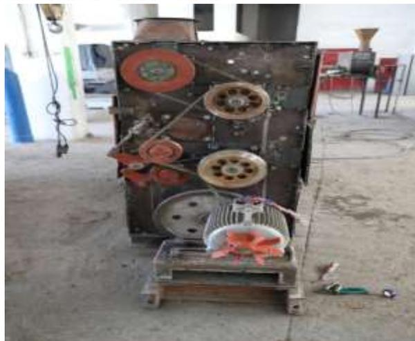
Fig.5. General view (drive) of the 2RKH-M regenerator.
