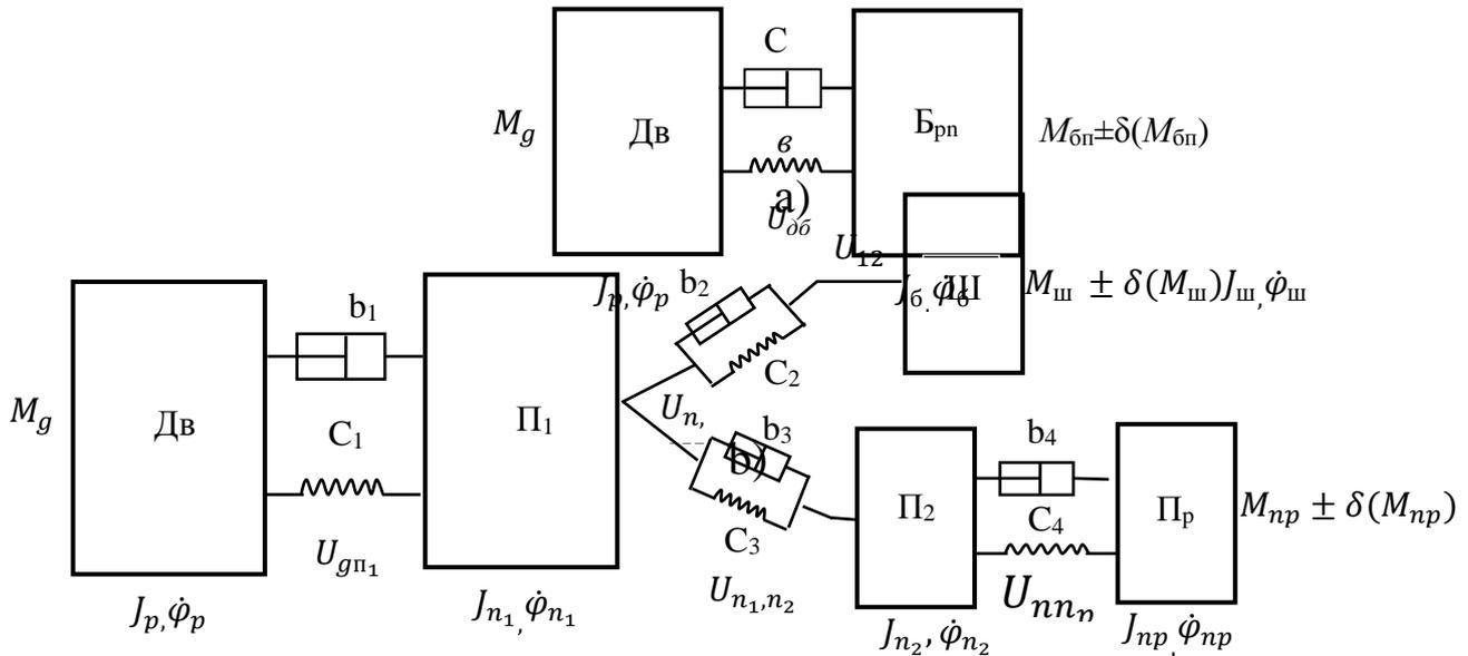
Fig. 2. Dynamic models of machine units with drive mechanisms of a rubber-slatted drum (a), saw bars and drums, as well as a impurity auger (b).
